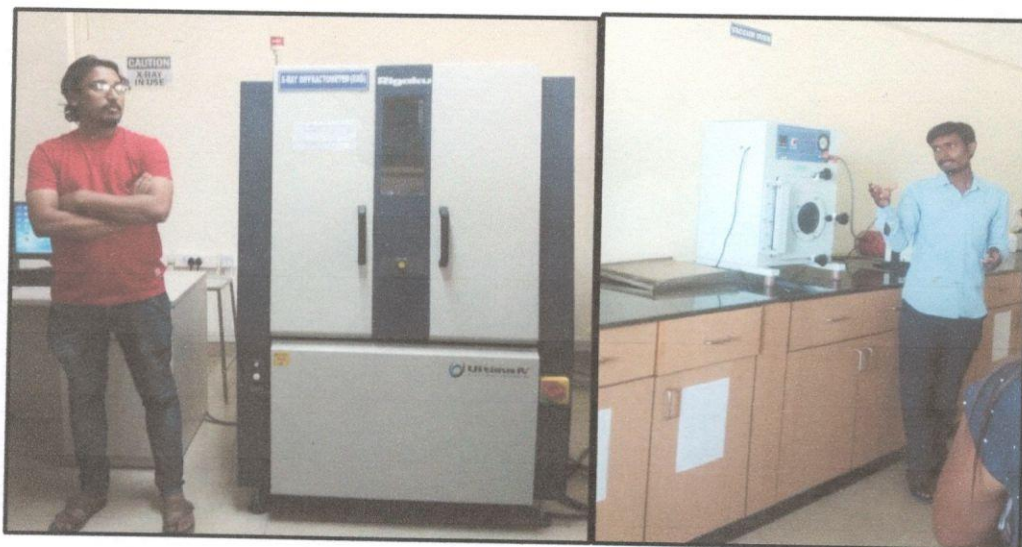
Left panel shows the X RAY diffractometer and the right panel shows equipment to synthesize nanomaterials under high pressure and vacuum.
